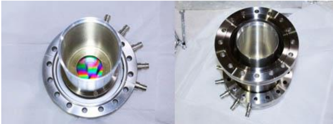
Figure 12 Output lens elements mounted on the detector assembly
