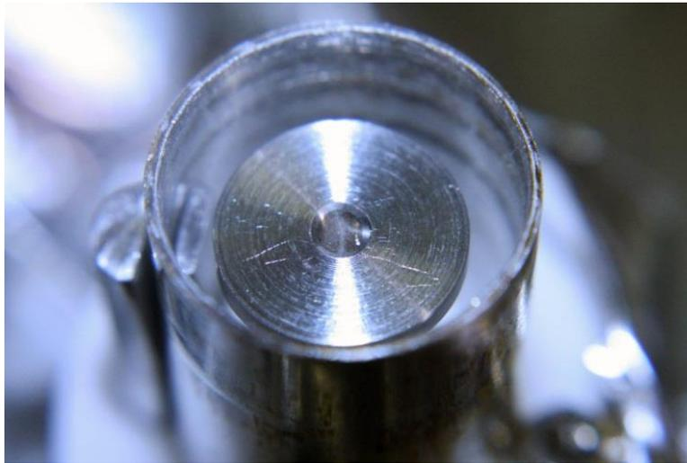
Figure 7 Au grid on sample stub
